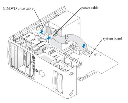
**4** Slide the drive release mechanism to the right to release the shoulder screw and slide the drive out to remove it from the drive bay.
